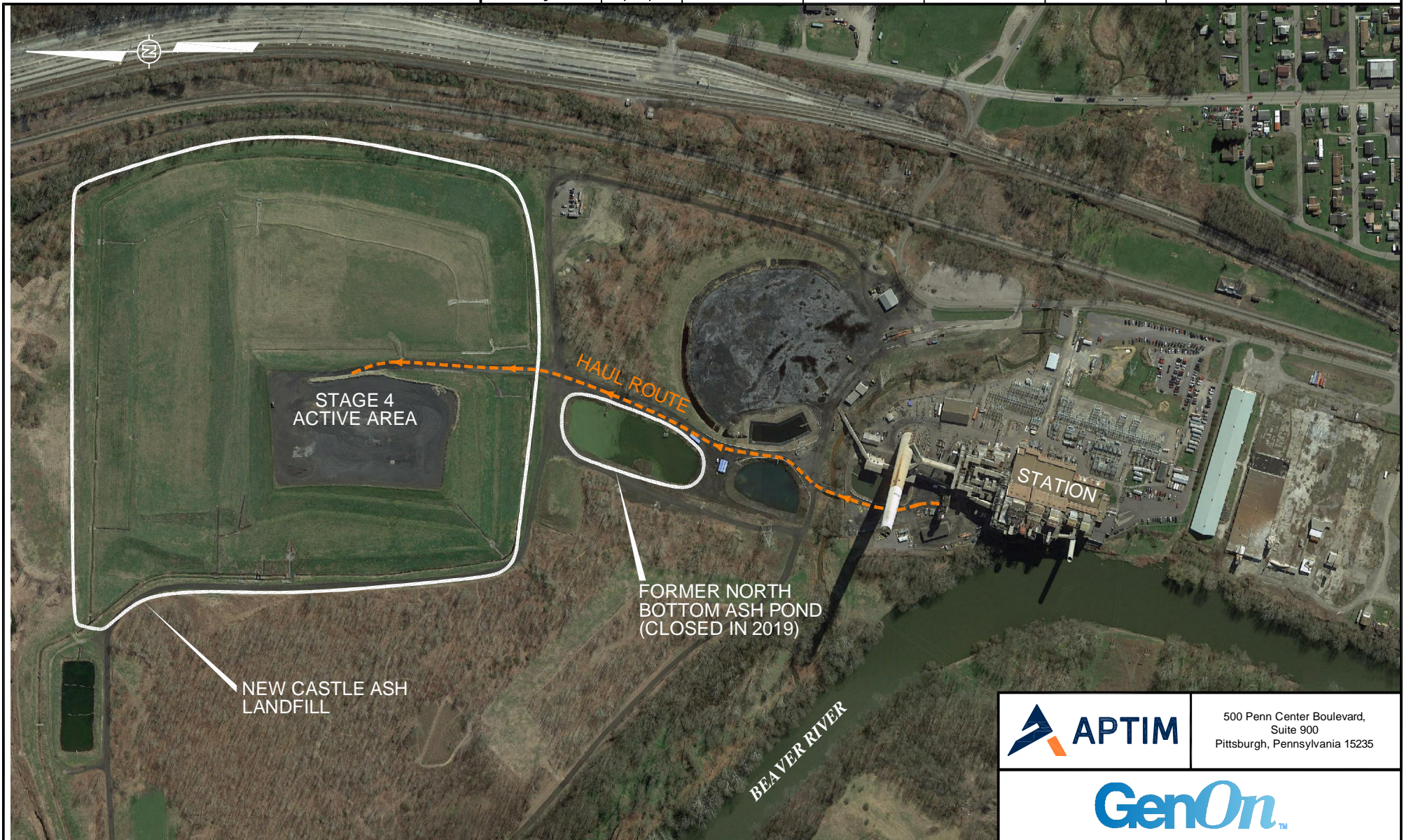
FIGURE 1 SITE LAYOUT AND POTENTIAL CCR FUGITIVE DUST SOURCES NEW CASTLE GENERATING STATION LAWRENCE COUNTY, PENNSYLVANIA
